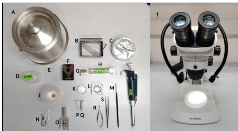
Figure 2. Materials Required for Adult Drosophila Muscle Dissection. (A) Liquid Nitrogen Container. (B) Slide Holder. (C) Petri Dish covered with Aluminium foil. (D) Ether in the dispensing bottle. (E) Glass Slide (F) Antifade Mounting Media. (G) Coverslip. (H) A vial containing wild-type flies. (I) Micropipette. (J) Etherizer. (K) Sylgard Plate. (L) Cavity Block. (M) Round Brush. (N) Razor Blade. (O) Transparent nail polish. (P, Q) Microfuge tubes for primary and secondary staining solutions. (R) Spring Scissors. (S) Forceps. (T) Zoom Stereo-Binocular Microscope. (Note: All required materials, including the reagents and fluorescence microscope, aren't shown).
